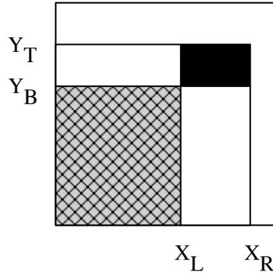
**Figure 2:** (after [Crow84]) An entry in the summed-area table holds the sum of the values from the lower left corner of the image to the current location. To compute the sum of the dark rectangular region, evaluate  $T[x_R, y_T] - T[x_R, y_B] - T[x_L, y_T] + T[x_L, y_B]$  where  $T$  is the value of the entry at  $(x, y)$
