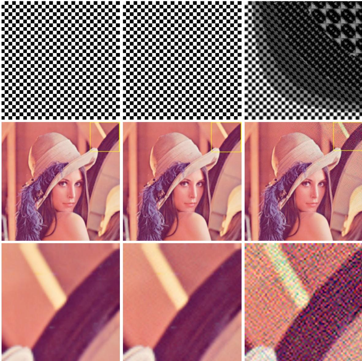
**Figure 4:** The left column shows the original input images, the middle column are reconstructions from summed-area tables (SATs) generated using our method, and the right column are reconstructions from SATs generated with the old method. For the first row, the SATs are constructed using 16 bit floats, for the second row the SATs are constructed using 24 bit floats, and the final row shows a zoomed version of second row (region-of-interest highlighted)
