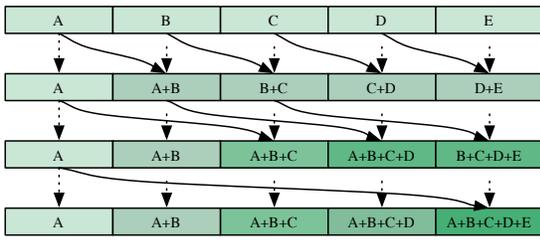
**Figure 3:** The recursive doubling algorithm in 1D. On the first pass, the value one element to the left is added to the current value. On the second pass, the value two elements to the left is added the current value. In general, the stride is doubled for each pass. The output is an array whose elements are the sum of all of the elements to the left, computed in  $O(\log n)$  time.
